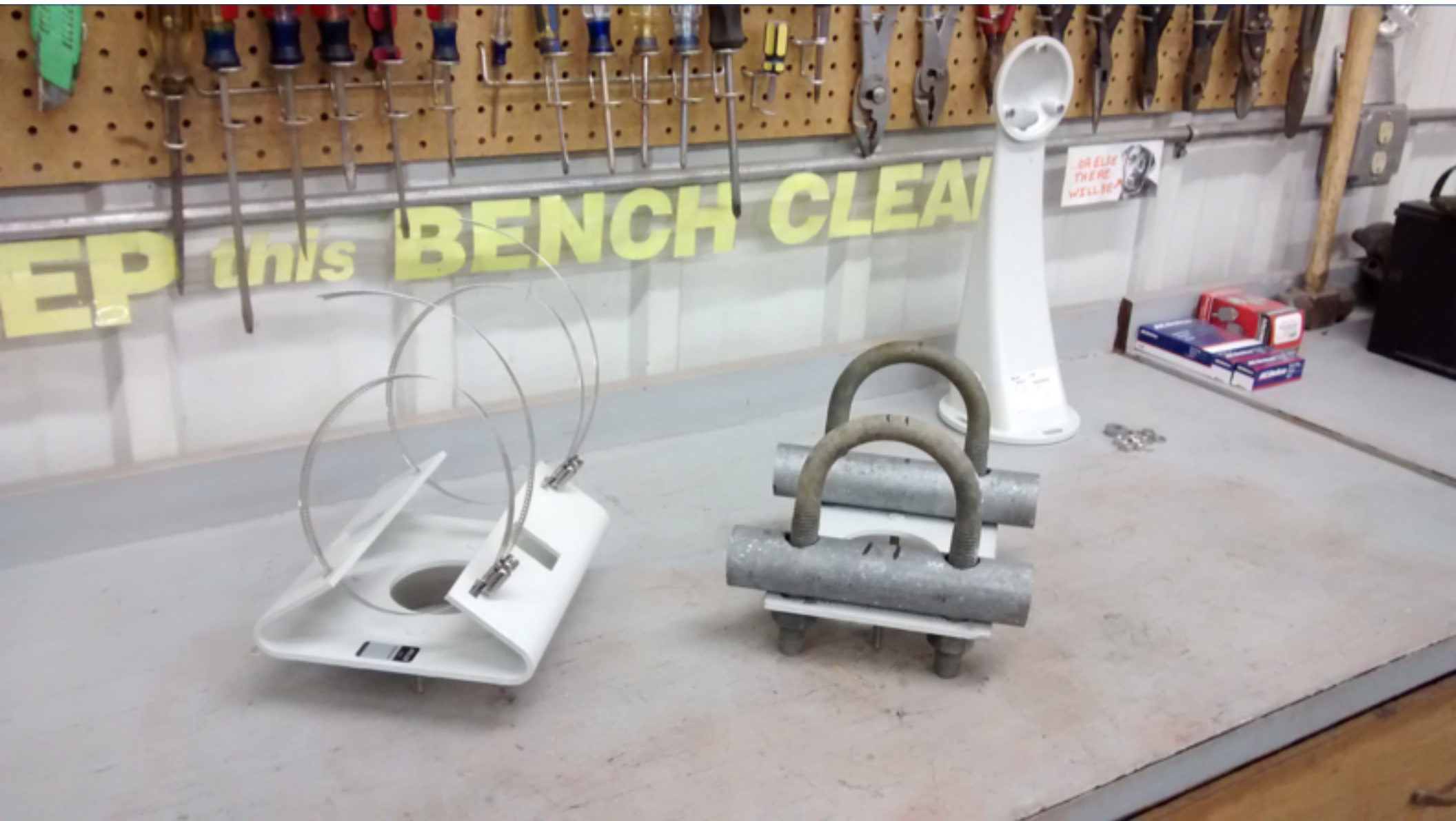
...such as this heavy-duty leg clamp (on right - "standard duty" factory piece on left)...
